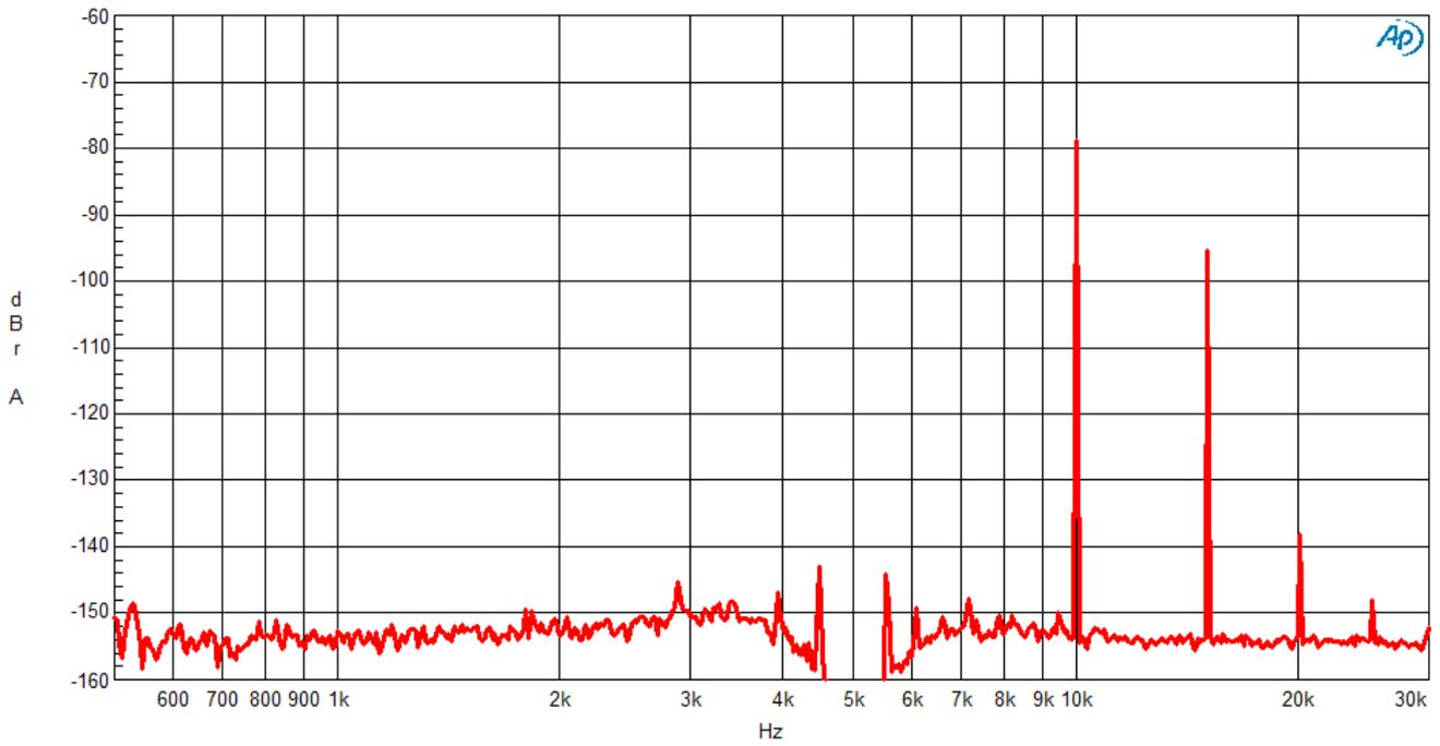
Fig.3 THD at 5kHz, 1V, balanced, 100k load
