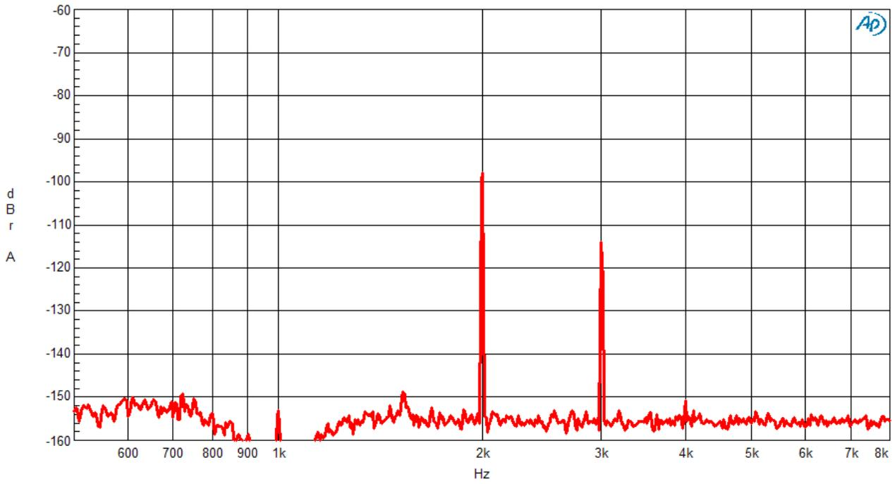
Fig.2 THD at 1kHz, 1V, balanced, 100k load
