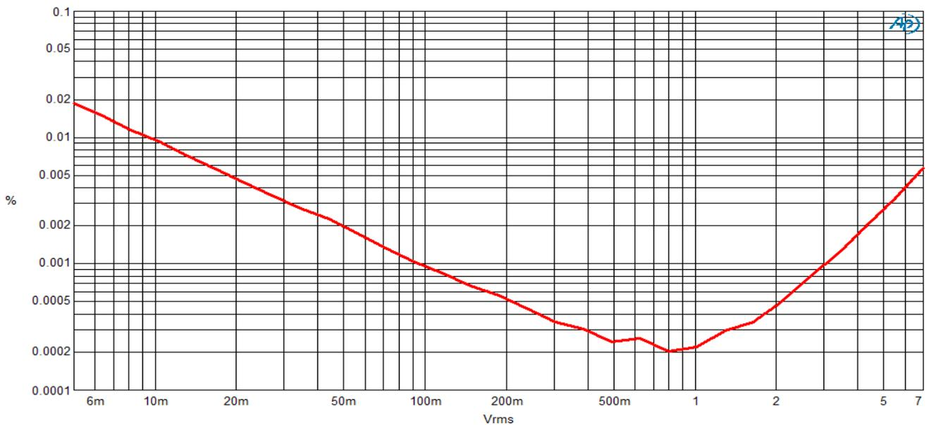
Fig.5 THD vs. level at 1kHz and 100k load
